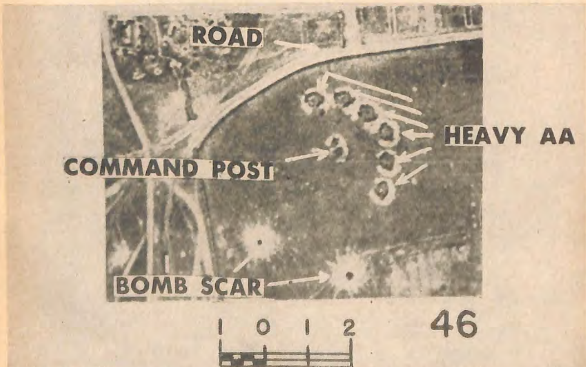
Figure 94. Six-Gun Heavy (105-mm) Antiaircraft Battery. Note shallow arc pattern with command post in center.
